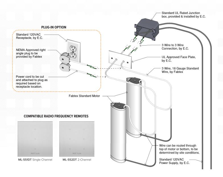
The motor produces less than 40bDA and operates on motorized track. Designed as a plug-in device for ease of installation, the plug can be discarded for hardwired installations. The included 12-foot power cord can be configured on-site to run on the bottom, side, or top of the motor. Available with wall or ceiling mount bracketry.
